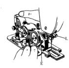
Slide Buttonholer in position from rear of Presser Bar, guiding Forked Arm Lever (L) over needle set screw. The Presser Bar of your sewing machine will fit into square groove of Buttonholer.
